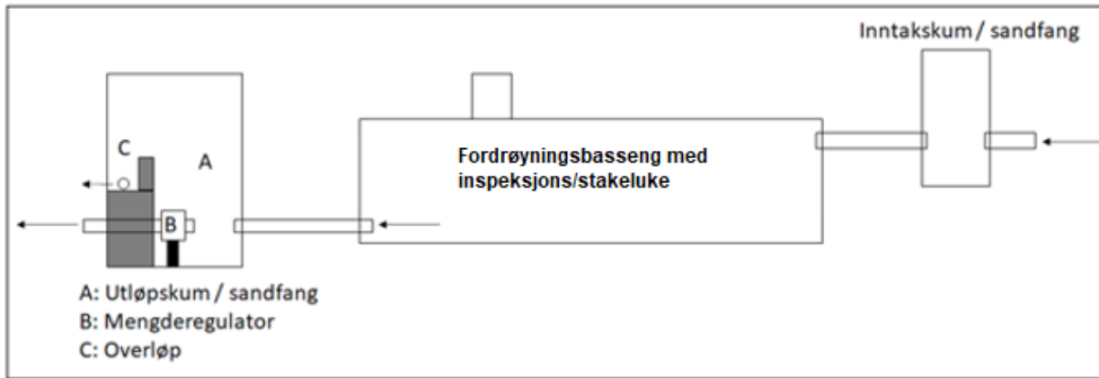
Figur 10: Prinsippskisse for fordrøyningsbasseng.
