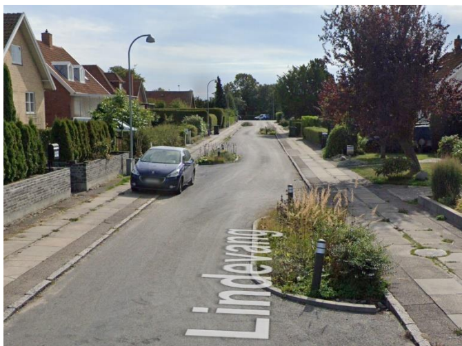
Figur 43: Regnbed langs veien Lindevang, Brøndby i Danmark (Foto: Google Steet view september 2022).
