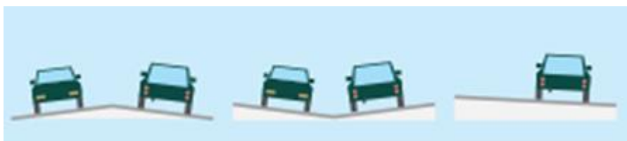
Figur 11: Ulike tverrprofiler (Figur: [23]).
